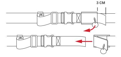
Following the research on quick release tethers from UCLan and adopting the same principle as our PFD chest harnesses, our waist belts are more adjustable and more reliable, eliminating the need to cut your belt to length. By separating the quick release and the waist adjustment buckle, the quick release tail is always the optimal length and the belt can be easily adjusted for people of all sizes with the spare webbing neatly coiled away.
